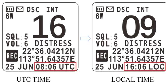
When the HM360 DSC MAX cannot receive the GPS signal to display the current position, the screen will automatic display the UTC local time and date.
